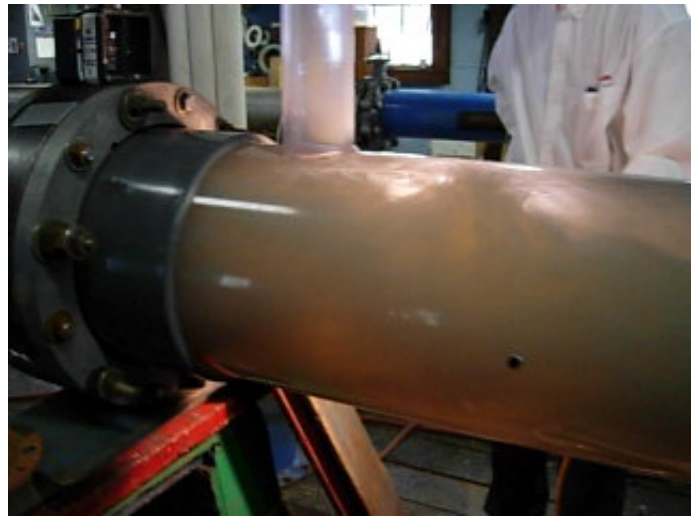
Figure 7 – End-of-Line Test, Enhanced plates, 50%open, air intake closed.
