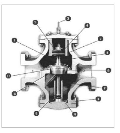
**Superior Features** Main valve is not subject to sudden failure. Piston movement is gradual and positive, preventing water hammer.
