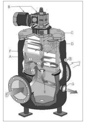
hollow port assembly not in contact with the screen surface. The drive shaft shall be supported at the top with permanently sealed enclosed stainless steel roller bearings in a double reduction gear reducer and water lubricated guide bearings at the bottom. Drive motors shall be 120/1/60 \_\_\_\_ HP, Nema 4, TEFC motor.
