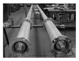
be continuous and full penetration. All torque tubes shall incorporate a permanent stainless steel tag with the maximum allowable torque to be applied to the assembly.
