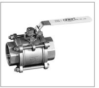
butt weld ends on ball valves. Swing out center body to accommodate inline maintenance. All valve seats are to be RPTFE. Stem packing is to be adjustable PTFE. All manual valves are to be supplied with Stainless Steel Locking levers and locating stops. All valves are to be designed to seal bubble tight at the rated pressure and low pressure. All valves shall be PMP A301 or reviewed equivalent.
