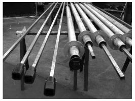
Pedestals shall be carbon steel epoxy coated in accordance with NSF 61 inside and out or 316 stainless steel. Pedestal bases shall be square and designed for a minimum of four mounting bolts. Mounting plate bolts shall be designed for one bolt to accommodate the total shear force based on the maximum design torque applied to the handwheel. All handwheels shall be a minimum of 300 mm (12 inches) in diameter.
